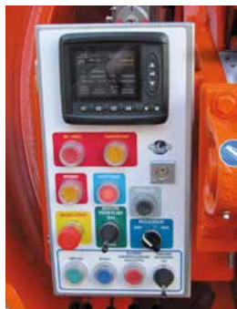
Rear control panel with IQAN display
